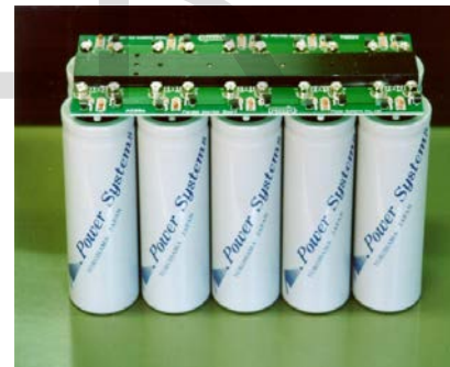
Fig 6: Photograph of a unit of 10 PSAP-8 EDLCs and parallel monitors
